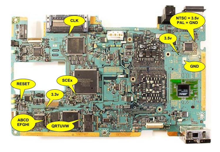
With reference to the above photo, solder wires to the **3.3v** and **GND** points. It is good practice to use thicker wire for power and ground and, of course, to insulate it.
