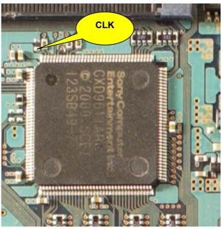
With the "easy" points now connected on the PS2 motherboard, you will need to solder the wires to the BIOS chip (points **MNOP QTUVRW**) and to the CD/DVD Controller (points **ABCDEFGHI**).
