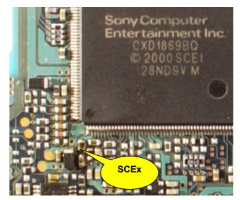
The **CLK** point is a pad above and to the left of pin 143 (see photo right). The **CLK** wire should be laid along the PS2 motherboard rather than allowed to run "in air". This is to ensure a proper ground plane to preserve the fidelity of the 36 MHz. Clock.
