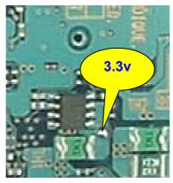
Install these points first. Note that **3.3v** & **GND** are 23 or 25 swg = 22 or 24 awg insulated stranded cable.
