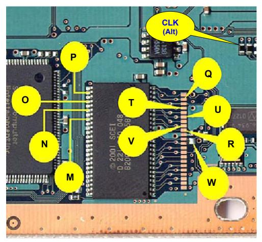
Points **QRTUVW** should be soldered first followed by **MNOP** which should traverse the BIOS chip and be secured to the top of the chip with Epoxy glue (lower photograph – please note this was taken before **W** was connected).
