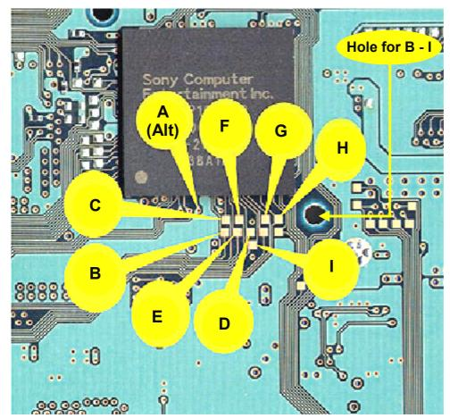
Turn the PS2 motherboard over. Locate the PS2 CD/DVD Controller pads (with reference to the schematic if necessary). Solder BCDEFGHI to the pads illustrated in the picture to the left.
