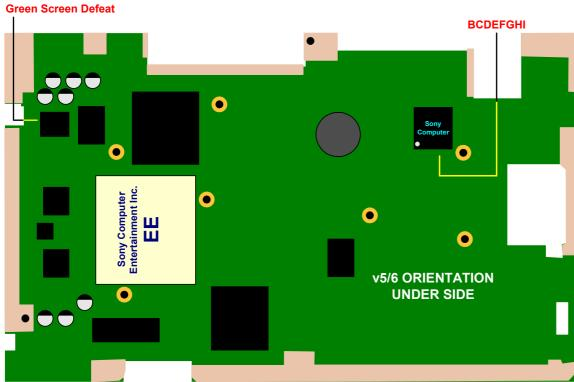
It is recommended that you solder to the PS2 motherboard first and then connect each wire to the appropriate point on the Messiah 2.
