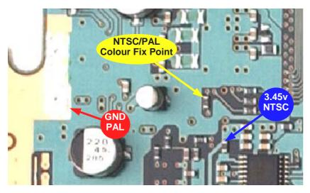
If you have an NTSC TV the Colour Fix point is taken to 3.45v. It forces NTSC colour on all PS2 game output. All PAL games will then be put out in NTSC colour mode and all PS1 games will display proper NTSC colour. The frame rate for PAL games will remain at 50 Hz.
