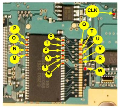
BIOS points **QRTUVW** should be soldered first (to the pads or to the legs according to your preference) followed by **MNOP** which should traverse the BIOS chip and be secured to the top of the chip with Epoxy glue (lower photograph).
