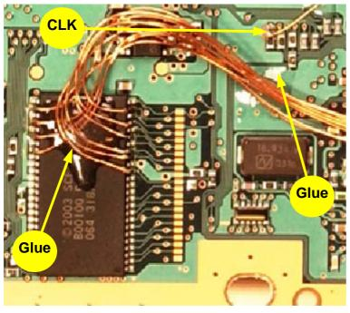
This completes wiring to the "top" side of the PS2 motherboard.
