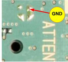
The GND copper pads are covered with lacquer that must be scraped off or the lacquer removed with flux spray as described in the soldering section.
