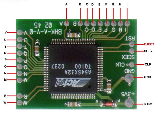
The v9 PS2 (SCPH 5000x) differs from its v7/v8 predecessors in that there are no convenient pads for the CD/DVD Controller (points **B-I**).
