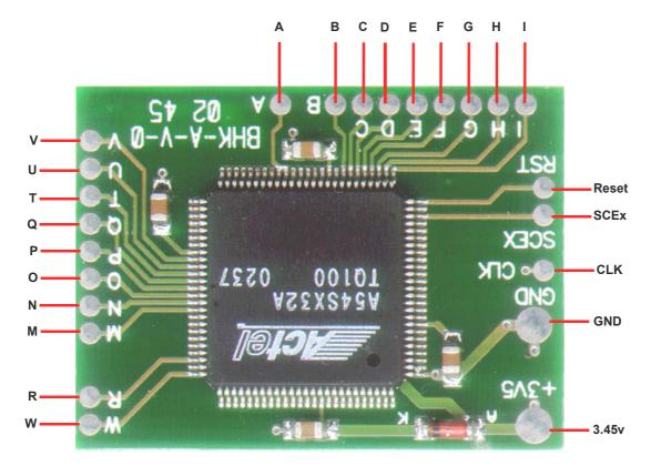
The schematics below show which PS2 motherboard chips are directly affected by the installation process together with their orientation on the motherboard. This covers points B, C, D, E, F, G, H, I on the CD/DVD Controller and Digital Signal processor; M, N, O, P, Q, R, T, U, V, W on the BIOS chip.
