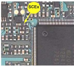
Now connect the **B** and **C** wires as per the photograph to the right and the **A** wire as per the photograph below. (**SCEx** is shown for positional reference).
