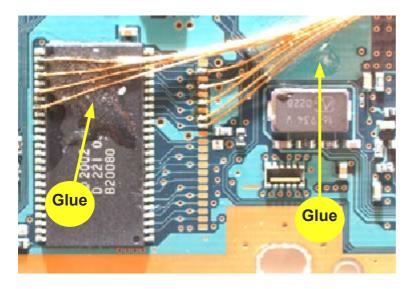
This completes wiring to the "top" side of the PS2 motherboard.
