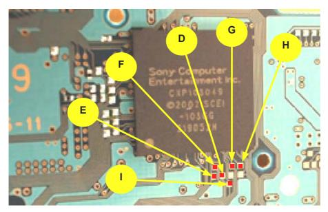
Turn the PS2 motherboard over. Locate the PS2 CD/DVD Controller pads (with reference to the schematic if necessary). Solder **DEFGHI** to the pads illustrated in the picture to the left.
