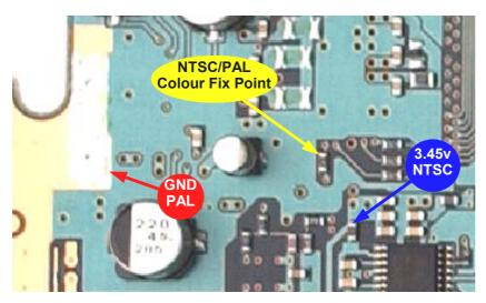
NTSC motherboards would require the *Colour Fix point* to be taken to 3.45v. It forces NTSC colour on all output. All PAL games will then be put out in NTSC colour mode and all PS1 games will display proper NTSC colour. The frame rate for PAL games will remain at 50 Hz.
