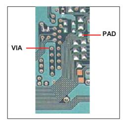
With reference to the picture on the left, it is straightforward to solder a wire to a **PAD**.
