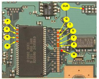
The **CLK** point needs to be carefully wired back to the Messiah 2. The wire should be laid along a ground plane – namely flat along the motherboard without traversing any surface mounted components.
